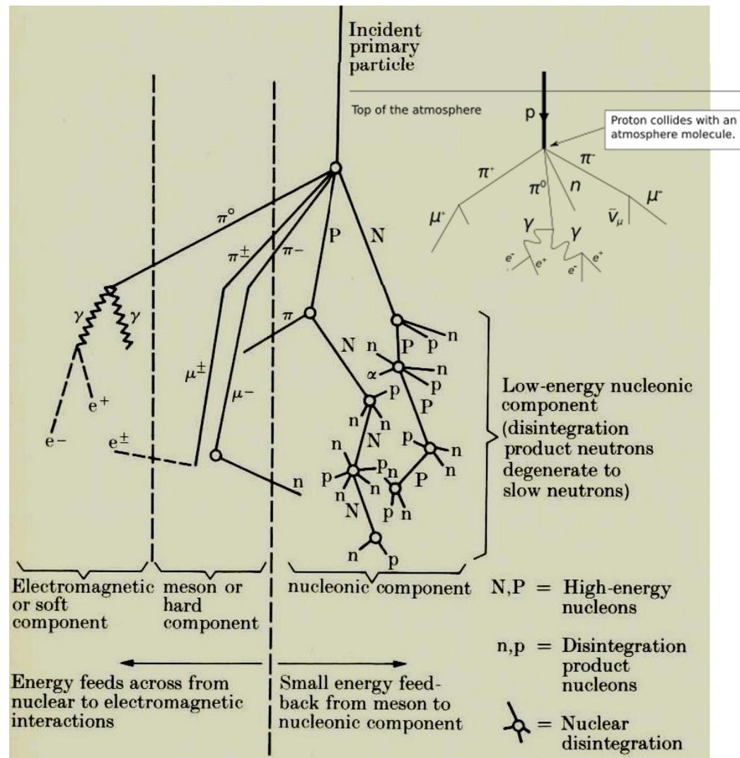
Fig. Interaction of the primary cosmic ray particle and the terrestrial atmosphere, resulting in secondary components of cosmic rays.
