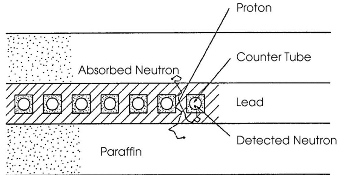
Fig. Schematic view of an IGY neutron monitor. The incident nucleon, here a proton, interacts with the lead. In the illustrated case three evaporation neutrons are produced in this nuclear reaction. In a random walk the neutrons travel in the different materials of the NM. Two neutrons are stopped in the reflector (absorbed neutron) and one evaporation neutron enters the moderator where it is slowed down, and finally it is detected in the counter tube.
