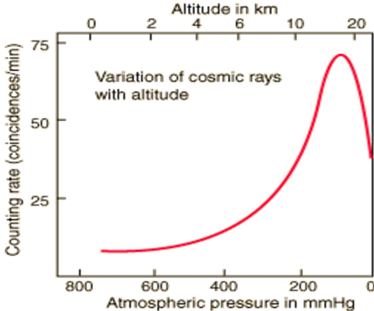
The detected cosmic ray flux peaks at about 15 km in altitude and then drops sharply (note the logarithmic scale on the altitude).
