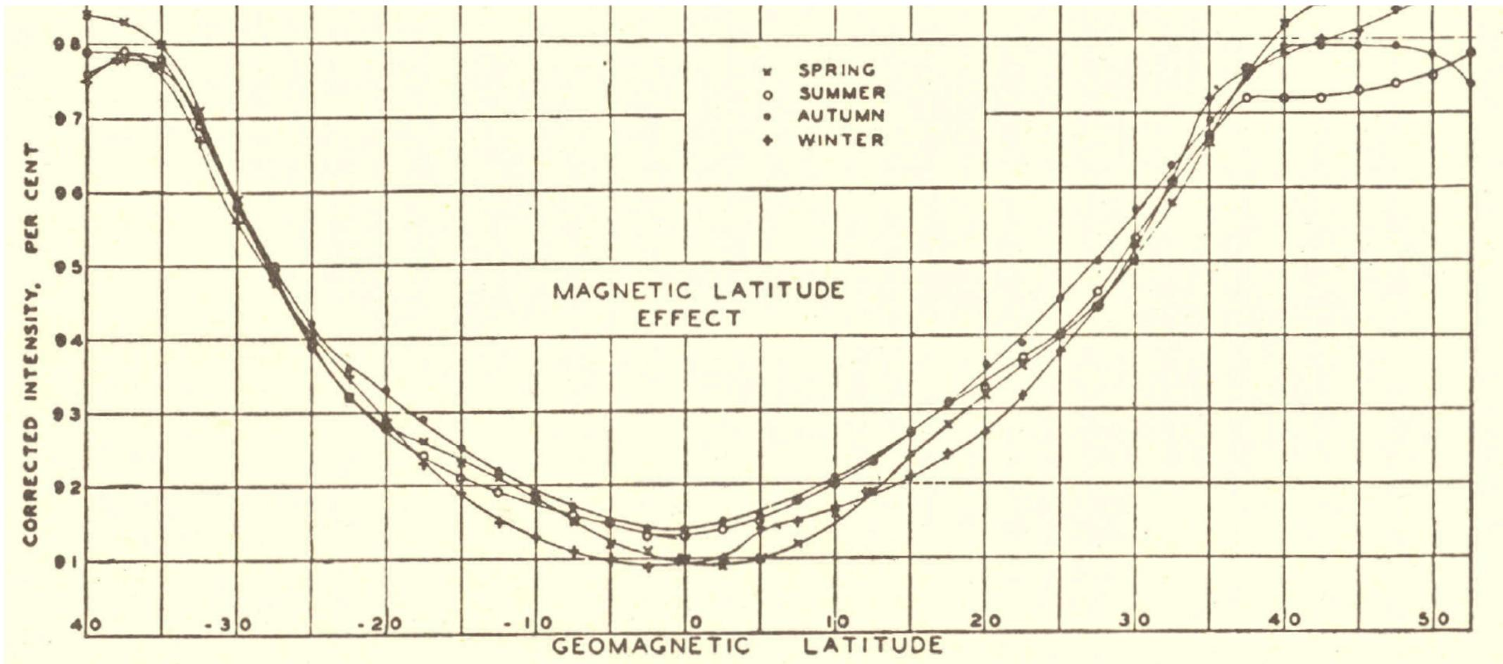
The intensity of **cosmic radiation** depends on **geomagnetic latitude** and **particle energy**.
