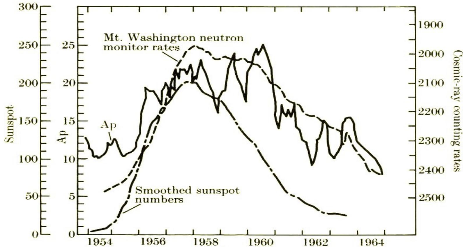
The level of the cosmic ray flux varies with solar activity - observed is eleven-year cycle variation of the cosmic rays. Because the solar activity varies significantly during the sunspot cycle, it is reasonable to expect that the interplanetary irregularities will also vary during the cycle, affecting the lower-energy cosmic rays much more than the higher-energy ones.
