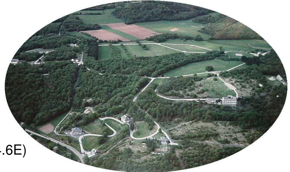
The Royal Meteorological Institute (RMI) Geophysics Centre at Dourbes (4.6°E, 50.1°N) is a complex observational site consisting of several observatories/stations – atmospheric, ionospheric sounding, cosmic rays, geomagnetic, GPS, etc.
