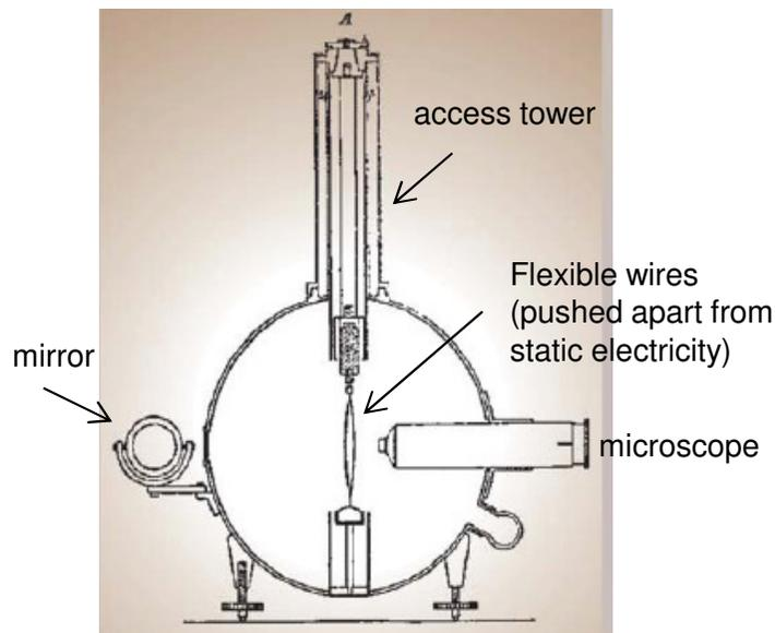
**Theodor Wulf's electroscope**, 1909. Shown is the instrument's 17-cm-diameter zinc cylinder with its pair of flexible wires below the access tower A. The wires are pushed apart by static electricity, and the microscope (peering in from the right) measures their separation, illuminated by light from the mirror at left. The air in the cylinder was kept dry by sodium in the small recess below the microscope.
